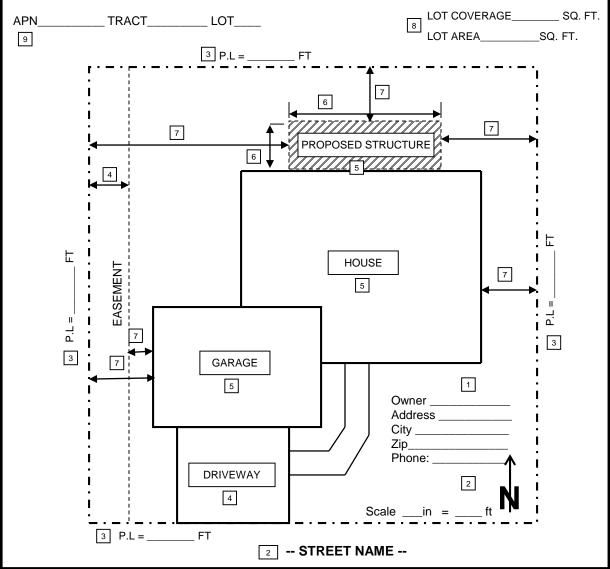
**INSTRUCTIONS:** Use this as an **example** to draw your own plot plan on a separate piece of paper. The following information is to be listed on your plot plan. Your plot plan must be uploaded with your application in the Carson Civic Access Portal.
